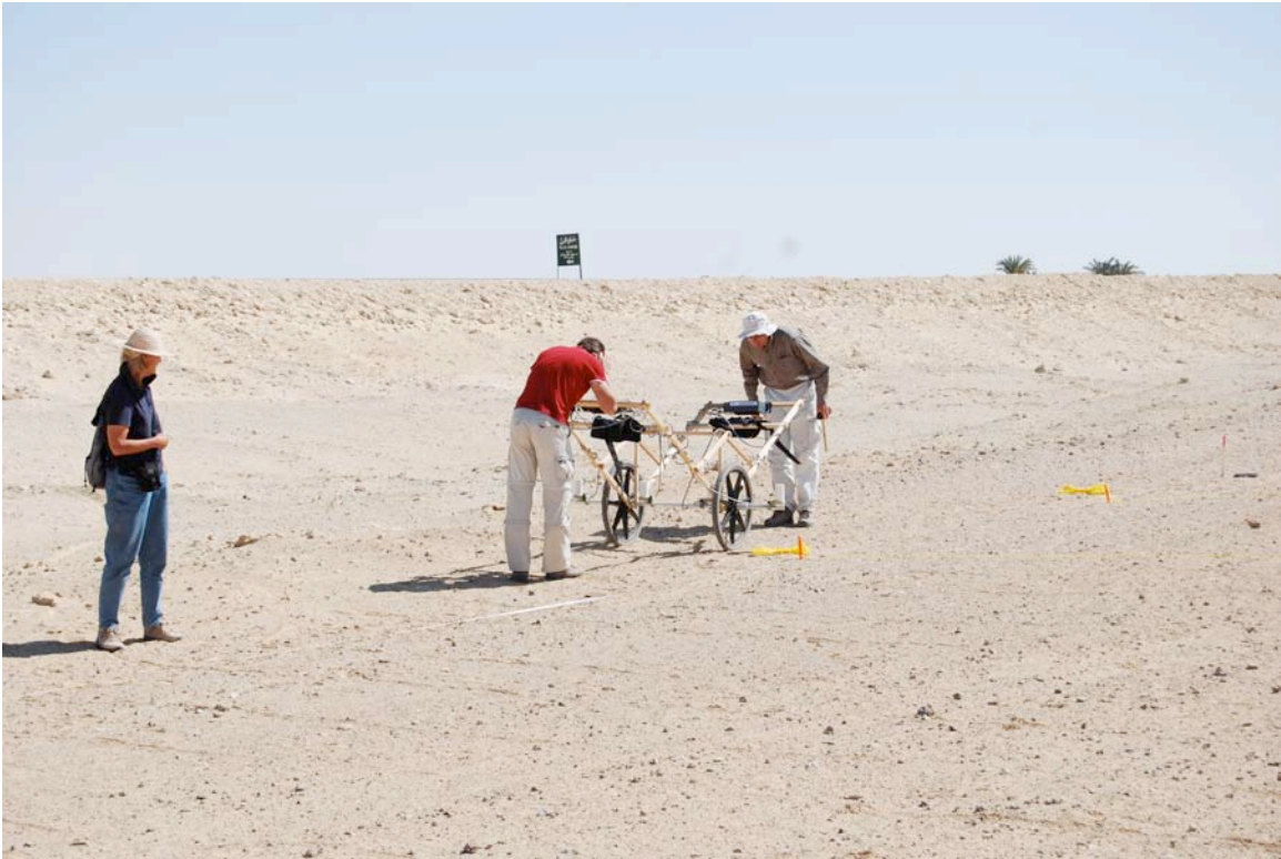
Fig. 5: Al-Zaytun. Magnetometer Geoscan G-858 with 4 sensors.
